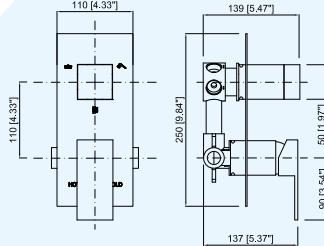
Thermostatic shower to build, ceramic diverter 3 outlets
